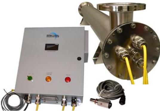
The electropolished, 316L stainless steel UV Reactor houses more lamps per volume of flow than MP. This provides a more uniform UV intensity field and inherent degree of redundancy. Consider the situation where a single lamp fails in a 2-lamp MP system versus an 8-lamp amalgam lamp system.
