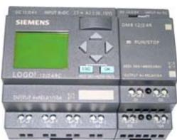
A standard Industrial Programmable Logic Controller (PLC), controls, monitors and reports the operating status of the UV System
